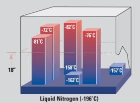
Mechanically Refrigerated Cryogenic Freezer
